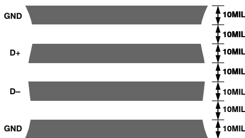
Figure 34. Arrangement of Signal Tracks
