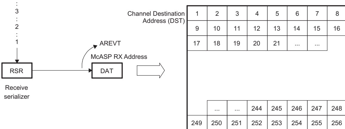
Figure 11-27. Servicing Incoming McASP Data Example PaRAM Configuration
